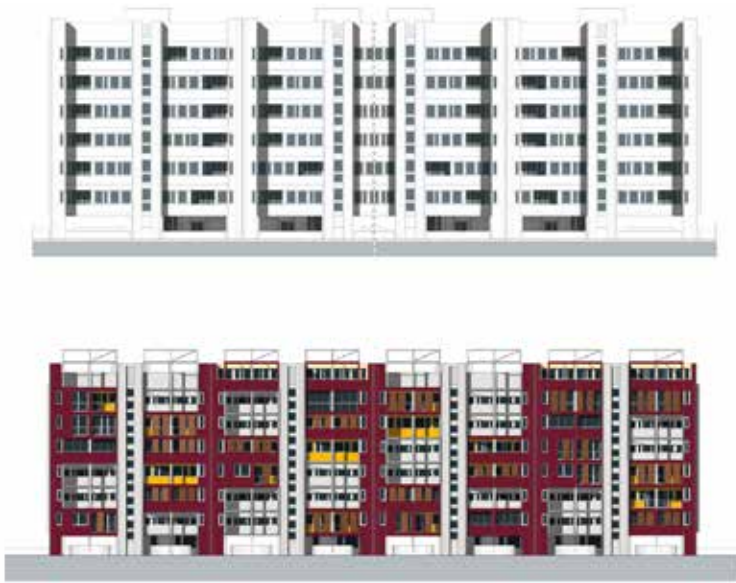
Fig.3 Building in via Goethe, PEEP Corticella. Elevation before and after, showing one of the possible facade combination that could result from the application of the proposed method.
